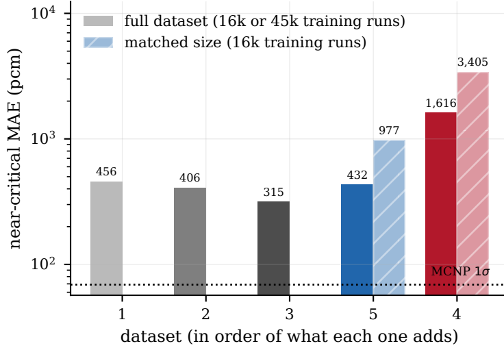
Figure 1: Near-critical mean absolute error up the complexity ladder, on each dataset’s locked test set. Solid bars use the full dataset; hatched bars repeat series 5 and 4 with the training set cut to 16,000 runs, the same as series 1–3. The dotted line is the median MCNP standard deviation, 69 pcm, the floor set by the labels themselves. Note the logarithmic scale.
