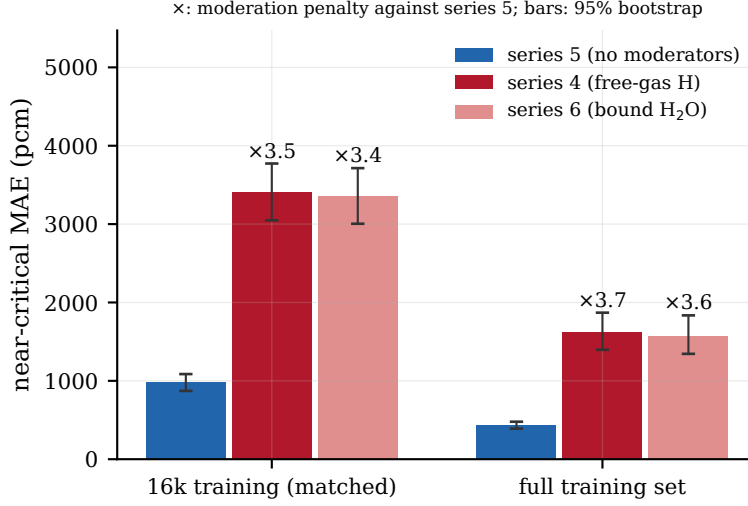
Figure 9: The moderation penalty with and without thermal-scattering data. Near-critical MAE on the locked test sets for the series-5 control, series 4 (hydrogen treated as a free gas) and series 6 (the same configurations with bound hydrogen in water), at the matched training-set size and at full size. Error bars are 95% bootstrap intervals; the multipliers are each dataset’s penalty against series 5. Correcting the labels leaves the penalty unchanged at both sizes.
